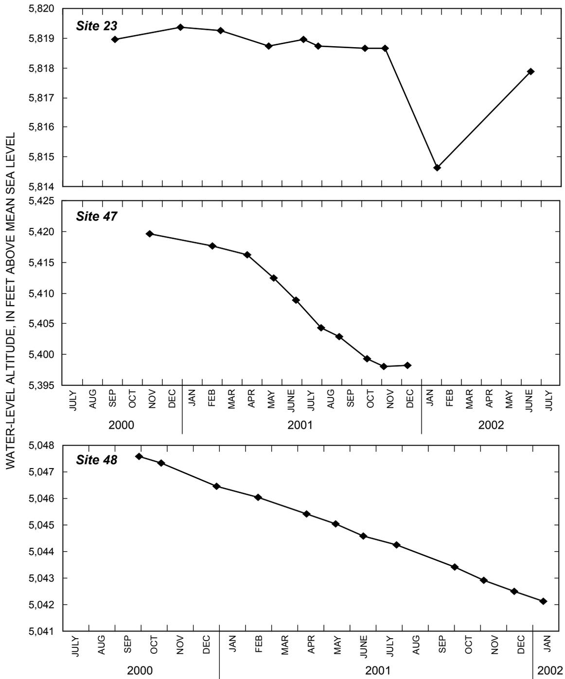
**Figure 9.** Measured water-level fluctuations in selected wells completed in consolidated-rock aquifers in the mountain block, 2000–2002, Tracy Segment Hydrographic Area, west-central Nevada.
