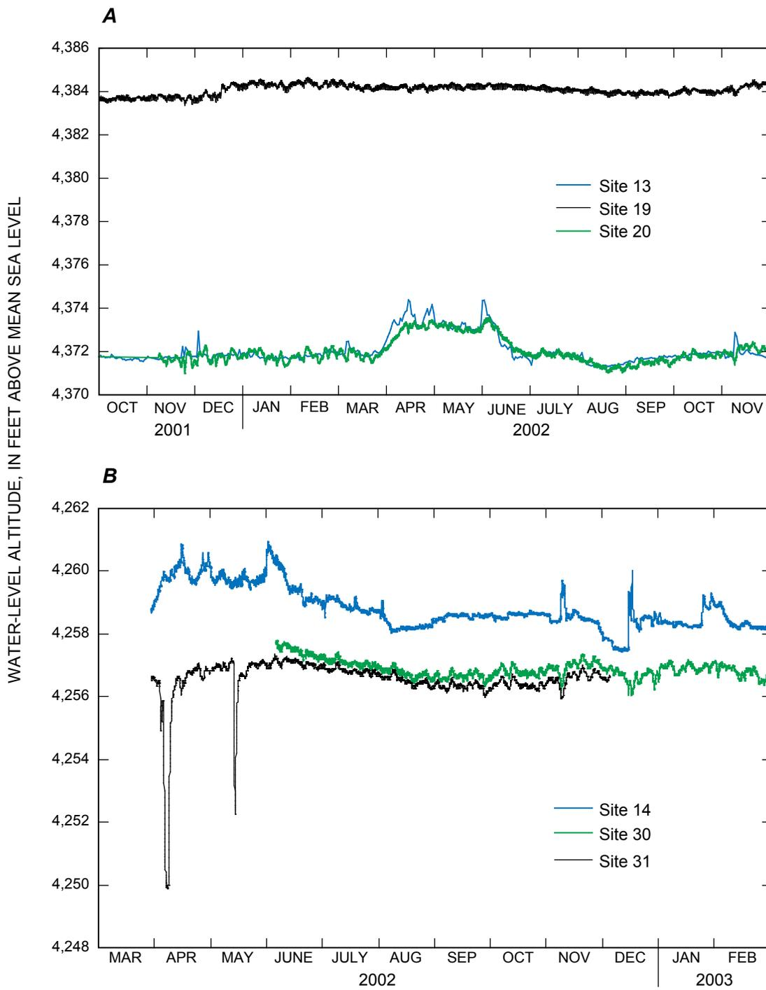
**Figure 11.** Relation between water-level fluctuations in nearby wells and Truckee River stage measured at U.S. Geological Survey streamflow-gaging station at Site 13 and near Site 14 (table 1), Tracy Segment Hydrographic Area, west-central Nevada.
