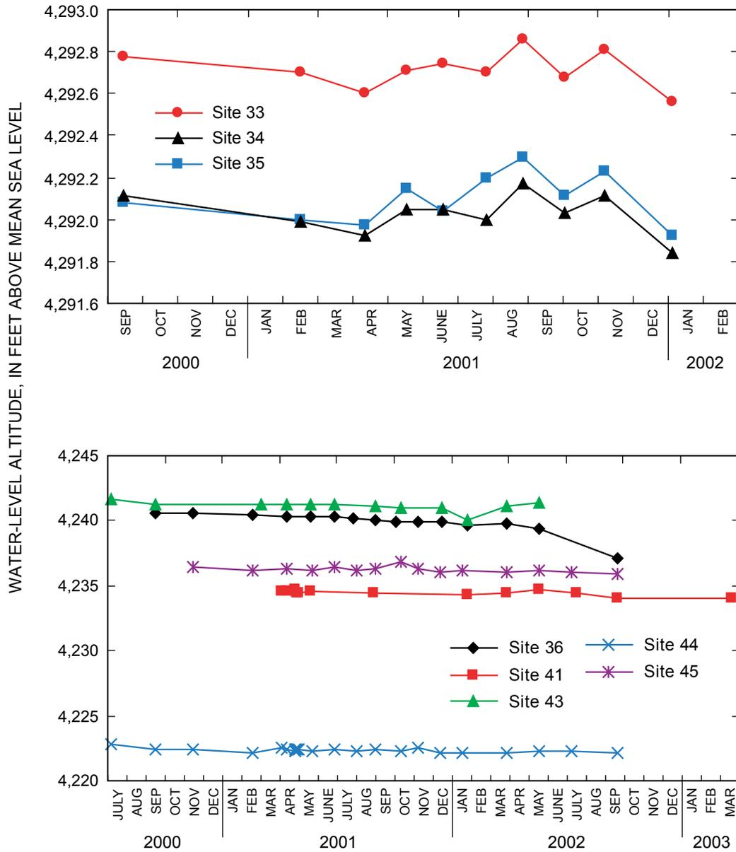
**Figure 10.** Measured water-level fluctuations in selected wells completed in consolidated-rock aquifers beneath alluvial-fan deposits, 2000–2002, Tracy Segment Hydrographic Area, west-central Nevada.
